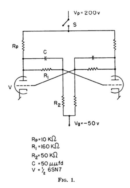
In this way we may obtain a finite random series of A and B which are statistically independent. One series produced by the aid of a flip-flop is given below:
