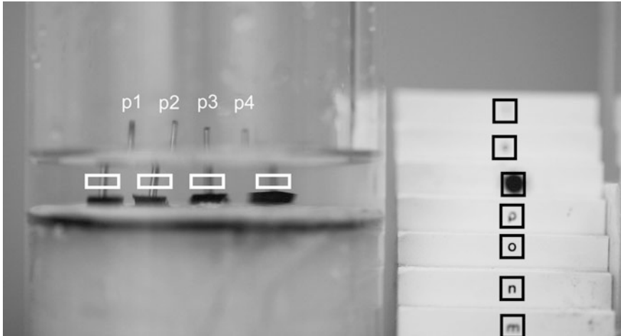
Fig. 16 Selected ROIs from acquired frontal images for analysis. The white rectangles are ROIs for each metallic pin ( p1 , p2 , p3 and p4 ) bellow water level. Black rectangles define ROIs for each focus stair step ( m , n , o , p , r —reference circle, s , and t )
