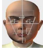
Fig. 3. The extracted features (gray points), the measured dimensions (gray lines) and the regions (orthogonals) of the face
