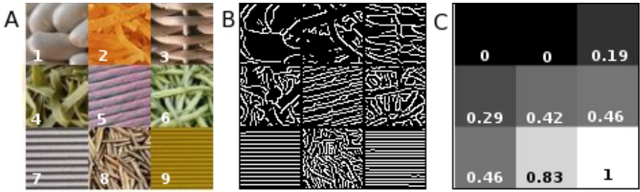
Fig. 2. Results for a mosaic image: (A) original mosaic image (B) edge map of the original images (C) presence degree of fineness textural concept obtained with the proposed model
