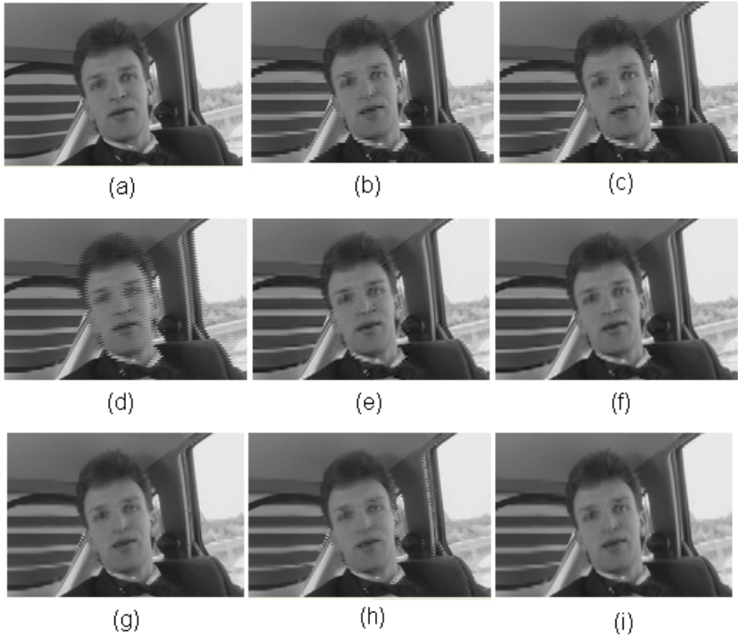
Fig. 3. (a) Progressive frame of 'Carphone' sequence. De-interlaced image applying: (b) line doubling, (c) line average, (d) field insertion, (e) 2-field VT filtering, (f) 3-field VT filtering, (g) fuzzy motion adaptive in [7], (h) proposal with 2 rules and (i) proposal with 3 rules.
