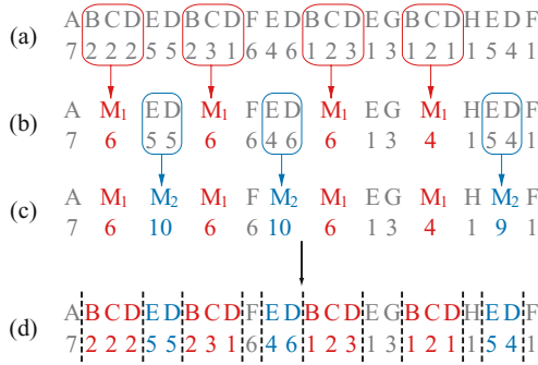
Fig. 3. Recursive motif extraction: (a)an original label sequence, (b)extracting the first motif, (c)extracting the second motif, (d)final segments
