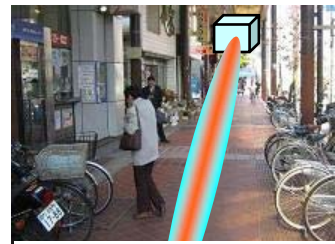
Fig. 4. A safe path between two rows of bicycles which makes Braille block not to work
