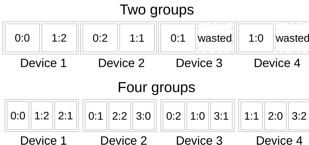
Figure 6.2: Data arrangement of groups with 3 components each. With only 2 groups 25% of capacity is wasted. With the number of groups increased to 4, the capacity is fully utilized.
